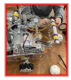
We finished removing all the mechanisms from last season. While removing the mechanisms we talked about the different options that are available for us to use. After completing our discussion we decided to add a motor with a green intake wheel to the back of the robot to move the
