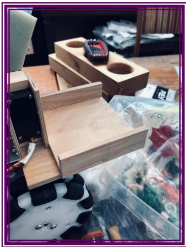
The tray and servo box are made out of 1/4 pine plywood. The plywood is better to use than solid pine because the plywood will not warp as much as the solid wood will.
